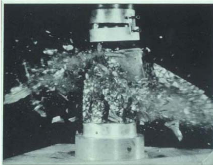
A cylinder of high-strength concrete is tested to failure.
