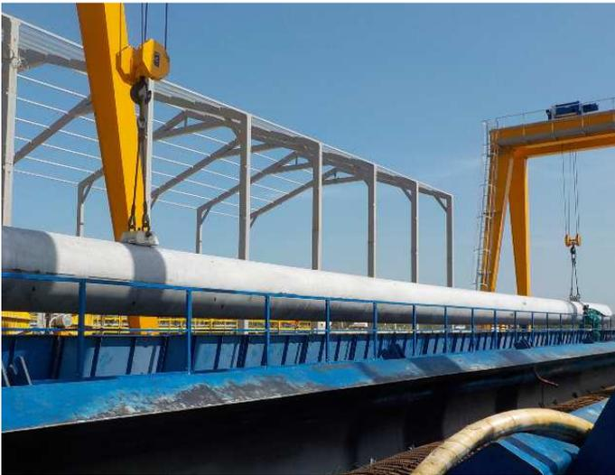
Figure 9. Pile de-moulding by means of gantry cranes / Scassero del palo mediante le gru a portale.
