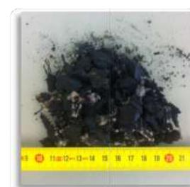
Figura 1 - Gomma G1:2-4mm      Figura 2 - Gomma G2:3.6-16mm
