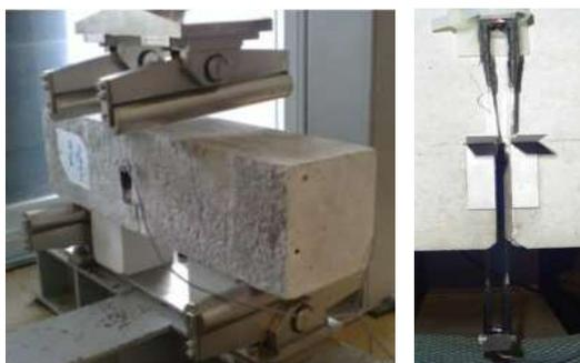
Figura 2 – Set-up prova UNI 11039
