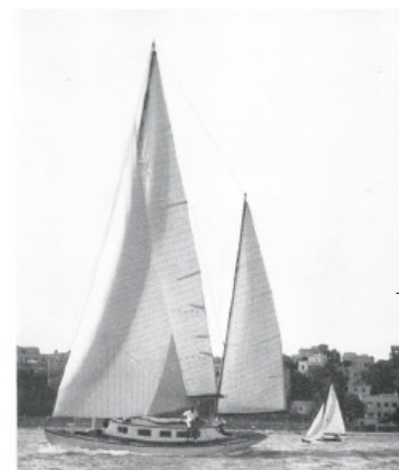
Ketch "Nennele" in ferrocemento
